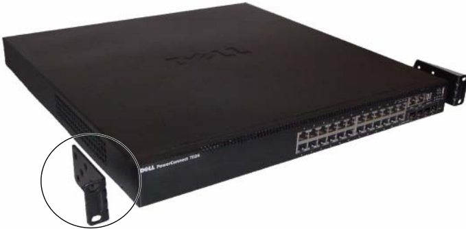
Figure 1-11. Attaching the Brackets
