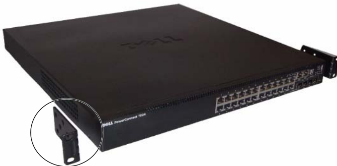
Figure 1-11. Fixation des supports
